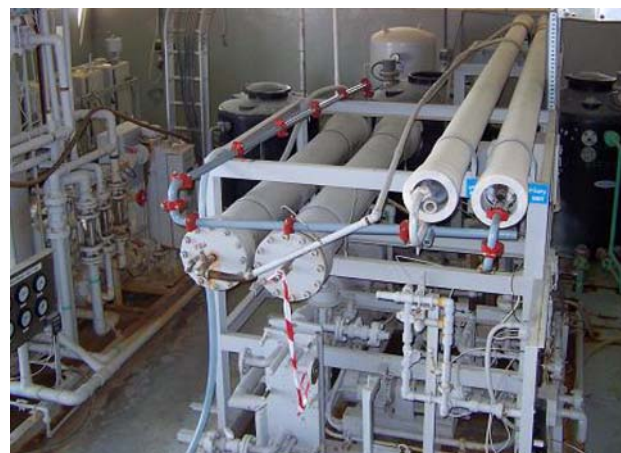
Fig. 1 Photograph showing the SWRO pilot plant test unit modified with thermoplastic piping
