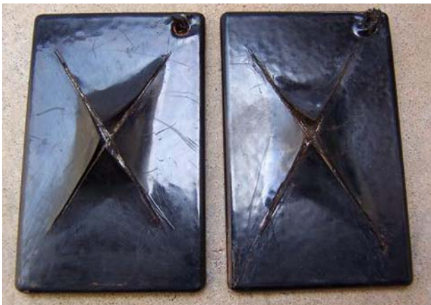
Fig. 4 Photograph of the coupons taken after 30 days of exposure in salt fog chamber. Loss of adhesion at the scribed mark can be seen
