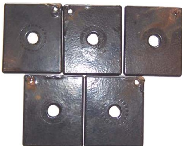
Fig. 6 Photograph of the coupons after crevice corrosion test in the laboratory. Absence of corrosion under crevice area can be seen
