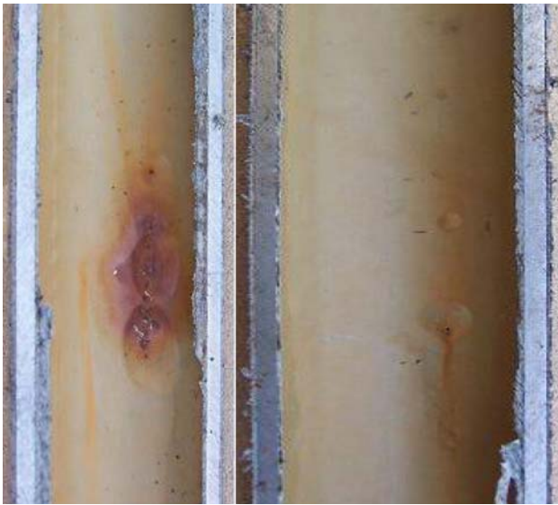
Fig. 3 Split view of the tubes showing blisters formation
