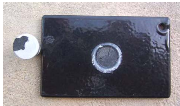
Fig. 7 Photograph showing the coated panel after pull-off adhesion test. A plug of coating detached from the substrate can be seen
